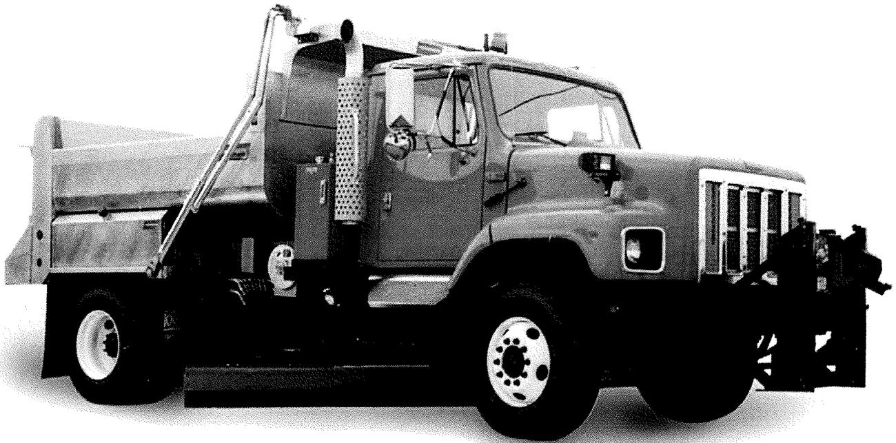
***Henderson Products, Inc. has yet another year round road maintenance product. This heavy duty underbody scraper features two double acting, power reversing cylinders for plowing angles up to 45 degrees. The 1" thick moldboard is available in 10', 11' and 12' lengths and is designed to provide superior winter snow and ice removal as well as summer road and shoulder grading***
